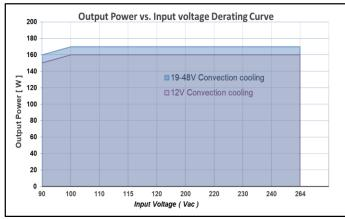
160W/170W Derate linearly 0.6% per Vac from 100 to 90Vac convection cooling at ambient temperature 40°C Max.
